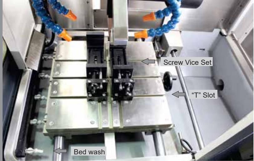
"T" Slot Bed: 600mm x 600mm with 12mm T-Slot
