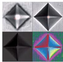
With software controlled focus, image cleaning, shading correction and regulated light source, reproducible results are obtained regardless of the number of indents measured. From perfectly polished to rough and etched samples, the auto-detection capabilities of WIKI 90 allow measurements on a variety of sample surfaces.
