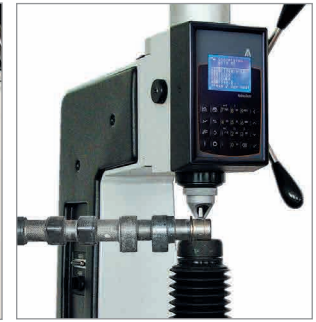
The visible penetrator permits testing in hard to reach areas (code 13606)
