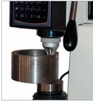
Clamping feature allows for testing large, overhanging parts without the need for additional fixturing
