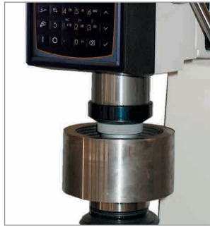
The 2 inch clamping stroke enables operations to clamp and test parts of various sizes in one easy motion without the need for height adjustments for easy of use and faster testing.
